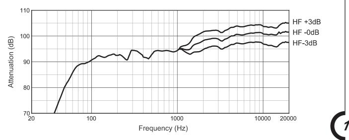
Below is an example of applying the ACS in a three-speaker array. In this particular configuration, the ACS on the top speaker is set at +3 dB, the middle speaker at 0 dB, and the bottom speaker -3 dB.
